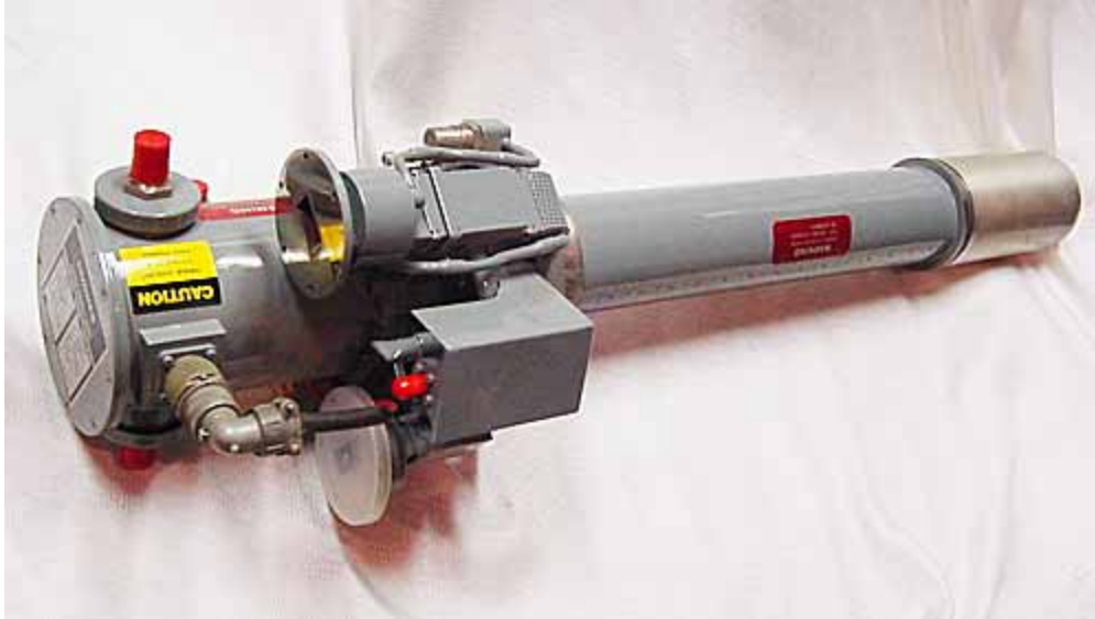
One example of Hughes EDD's High-powered Traveling Wave Tube from the 1970's
