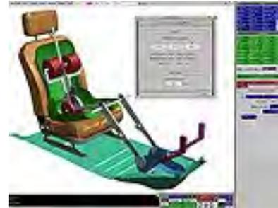
The Oasys HPM Positioning Tool provides an interactive environment to set-up and analyse the positioning of the H-Point Machine (HPM) in a seat.
