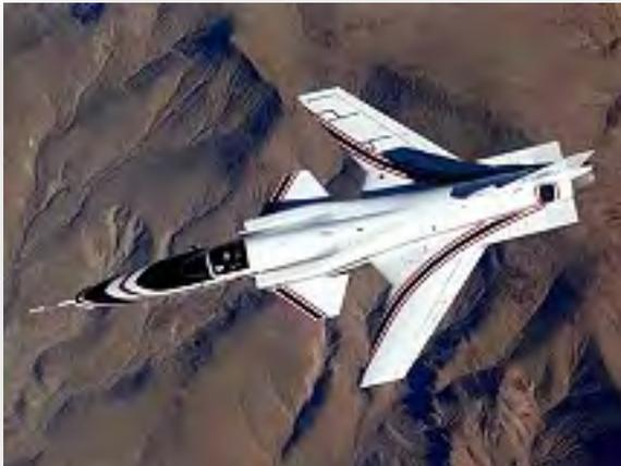
**This look-down view of the X-29 research aircraft in flight over California's Mojave Desert during the 1980s and 1990s shows its striking and unique forward swept wing and canard design.**
