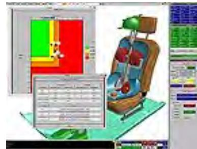
The Oasys HRMD Positioning Tool provides an interactive environment to set-up and analyse the positioning of the H-Point Machine in a seat and to assess the head restraint scoring.
